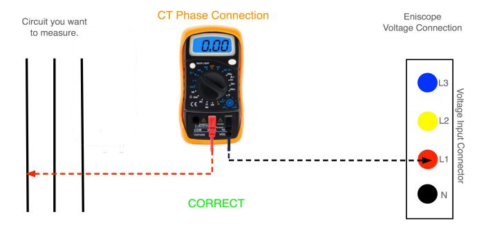
If however, you have a reading as below this shows you are measuring the potential between 2 different phases and proves you have the CT on the wrong phase. You can then simply move the second probe to the next phase until you get a zero reading indicating the correct phase and then place the CT on that phase.
