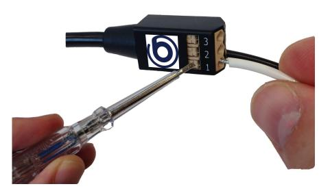
It's always important to check the device readings to confirm you have a correct installation.
