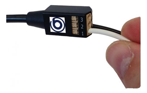
To remove the CT wire press firmly on the tab releasing the internal clamp and at the same time pull the cable.
