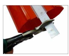
After cutting the extrusion, push the PCC until the next black cut line on the PCBA is exposed. Cut the PCBA on this next black cut line. This will allow the LEDs to illuminate up to this last black cut line. Not trimming the PCB to the last black line may cause some of the red LEDs to not illuminate.
