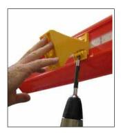
Push up on the screw until the bottom piece of the bracket is above the bottom track on the extrusion. Tighten the screw so the bottom piece of the bracket engages the bottom track of the extrusion. Tighten the screw until bottom piece of the bracket is firmly seated against the top piece of the bracket.
