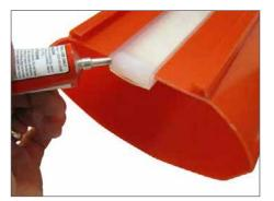
Use IPS Weldon #16 to bond a new end cap onto the cut extrusion. Put Weldon #16 around the entire end cap perimeter in all areas it will make contact with the extrusion. Put Weldon #16 around the entire perimeter of the cut extrusion including the small cavity where the PCBA is contained.
