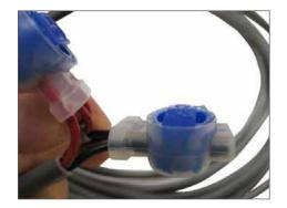
Make sure the wires are pushed all the way into the connectors so you can see them on the other side of the blue oval. Make sure the blue oval is fully depressed to make a secure electrical connection.
