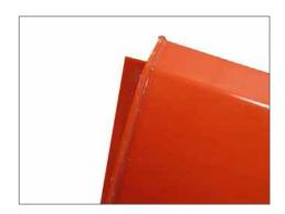
After bonding, inspect the joint to make sure there are no gaps. If a gap is seen, fill it with Weldon #16 and reapply pressure to that area for an additional 15 minutes. This seal is critical for keeping water out of the extrusion. Do not use Silicone on this seal. Silicone will not bond to the extrusion material.
