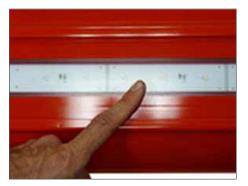
Gather materials: Sandpaper, Weld-On #16, silicone end plug, Humiseal 1B73 conformal coat (for sealing edge of LED board), and acrylic (field) end-cap. Cut the extrusion with a power miter saw (Chop Saw) at the desired length. Red Bar can be cut at any length measured from the end with the cable. (Cut off the end without the cable). The cut must be clean, straight and free of burrs. Remove any saw dust from the inside of the extrusion.
