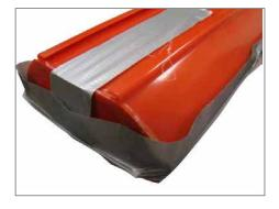
Press the end cap onto the extrusion and make sure it is aligned to cover the entire extrusion opening. **Apply even pressure to the end cap for at least 15 minutes**. Strong tape can be used to maintain pressure on the cap for the curing period.
