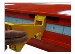
Hang the SRB section on the top piece of the brackets. The left photo above shows the SRB section on the two brackets at the ends. The right photo above shows the SRB section at the center bracket. Adjust the SRB section left or right by sliding it until it's in the desired location (pictures show brackets unmounted so track can be seen).
