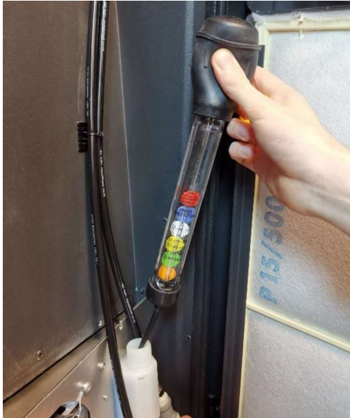
Figure 84: Check the coolant concentration using a refractometer
